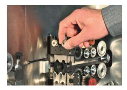
Rotary stripping technology can be integrated into a conventional cut and strip machine. Since the rotary stripping head can be programmed to make incisions at any depth into the insulation, this design eliminates the need for changing blades (radius blades, die blades, etc.) when processing different wire or cable sizes. While the production rate is somewhat slower, no blade changeovers
